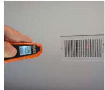
Item 26 - Item 3 (Picture) Sample supply temp. - Warm air in cooling mode
